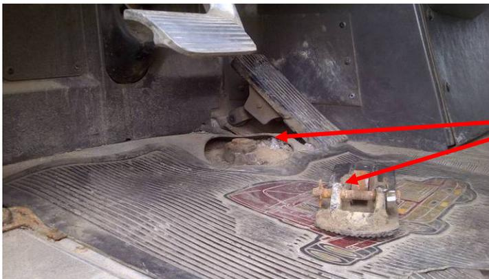
Broken Mounting Plate Ear / Pivot Support
