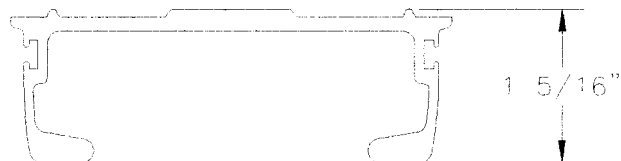
TYPE 35-2DS DECK SLAT 1.193 LBS. PER FT. PART NO. 41-3046
